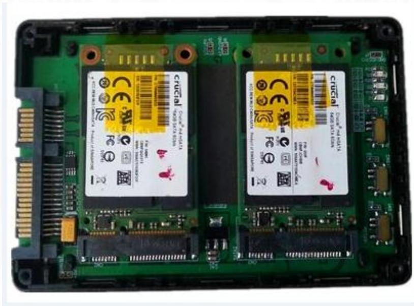
B: Connect SATA 15pin powered SSDMR directly to the computer.
